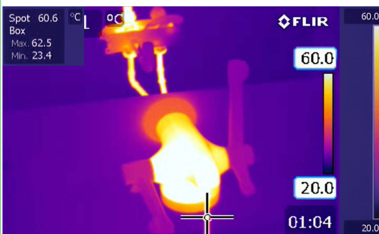
Thermal disinfection in-situ using the ILTDU
